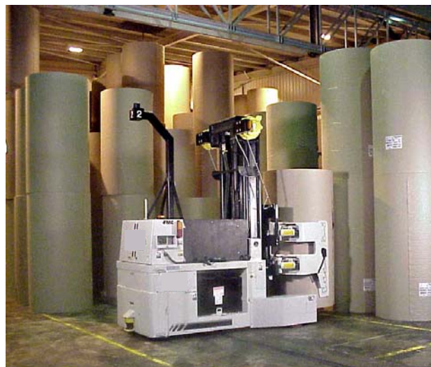
The equivalent clamp-model AGV uses precise positioning and pressure sensors to deliver just the right amount of force to ensure a safe grip.
